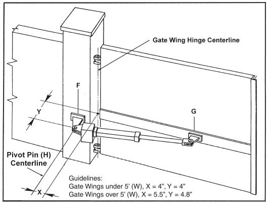
15. When the locations of the Arm Mounting Bracket (F) and the Pivot T-bracket (G) have been determined, mount the brackets with hardware (not supplied).
